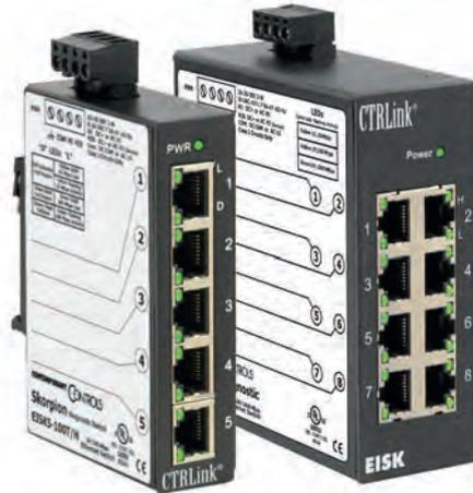
Instead of installing a managed switch with port-mirroring, the Skorpion Diagnostic Switch is often used at PlugFests, along with a sniffer tool like Wireshark to analyze BACnet messages sent over Ethernet. The Diagnostic Switch allows all participants at the PlugFests to connect at the data rate of their equipment with no concern for other participants' data rate. With the Skorpion Diagnostic Switch and a protocol tool, issues can be found in the development phase rather than in the field.
