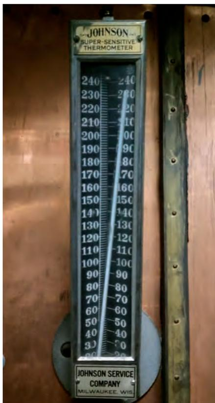
An old "Super-Sensitive Thermometer" by Johnson Service Company — the original name of Johnson Controls — on an air-conditioning unit. The glass capillary tube has come loose from its attachment and is leaning at an angle within the bezel.
