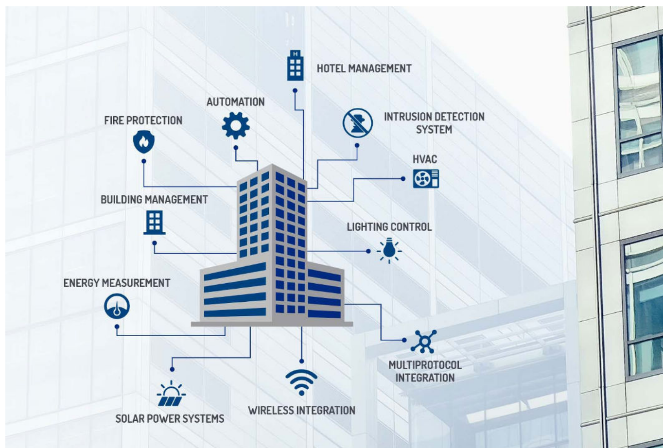
The integration problem: multiple systems providing services to the building users are not capable of communicating with each other by themselves. © HMS Industrial Networks, SLU
